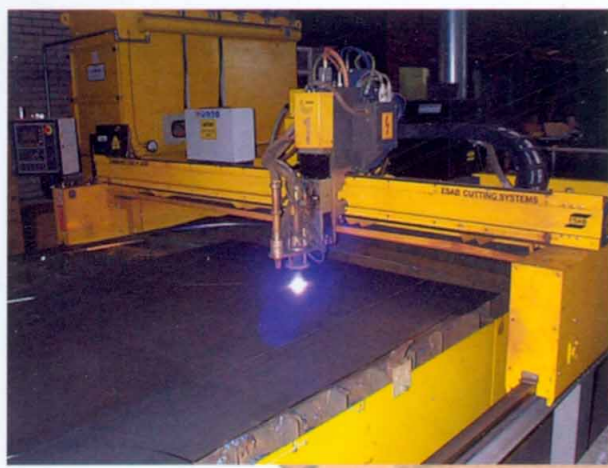
Reclaimer profiles are produced using a computer controlled plasma cutter.
