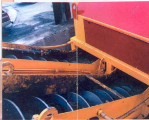
The sand is removed from the mix by sand screws.
