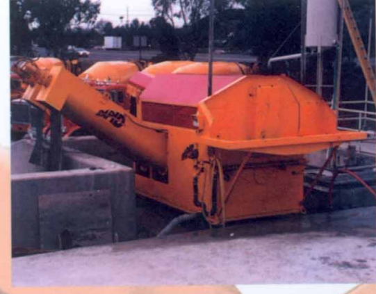
A MK2 Reclaimer set up between sand and aggregate pits and a settling tank.
